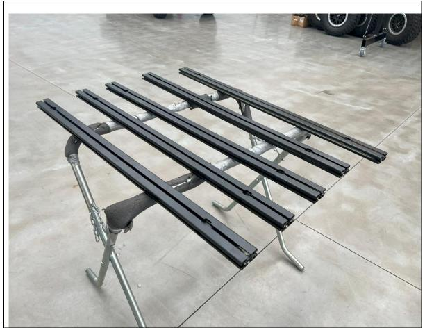
2. Next Assemble the roof rack. Start by setting out the 5 extrusions on a table or panel stand.
